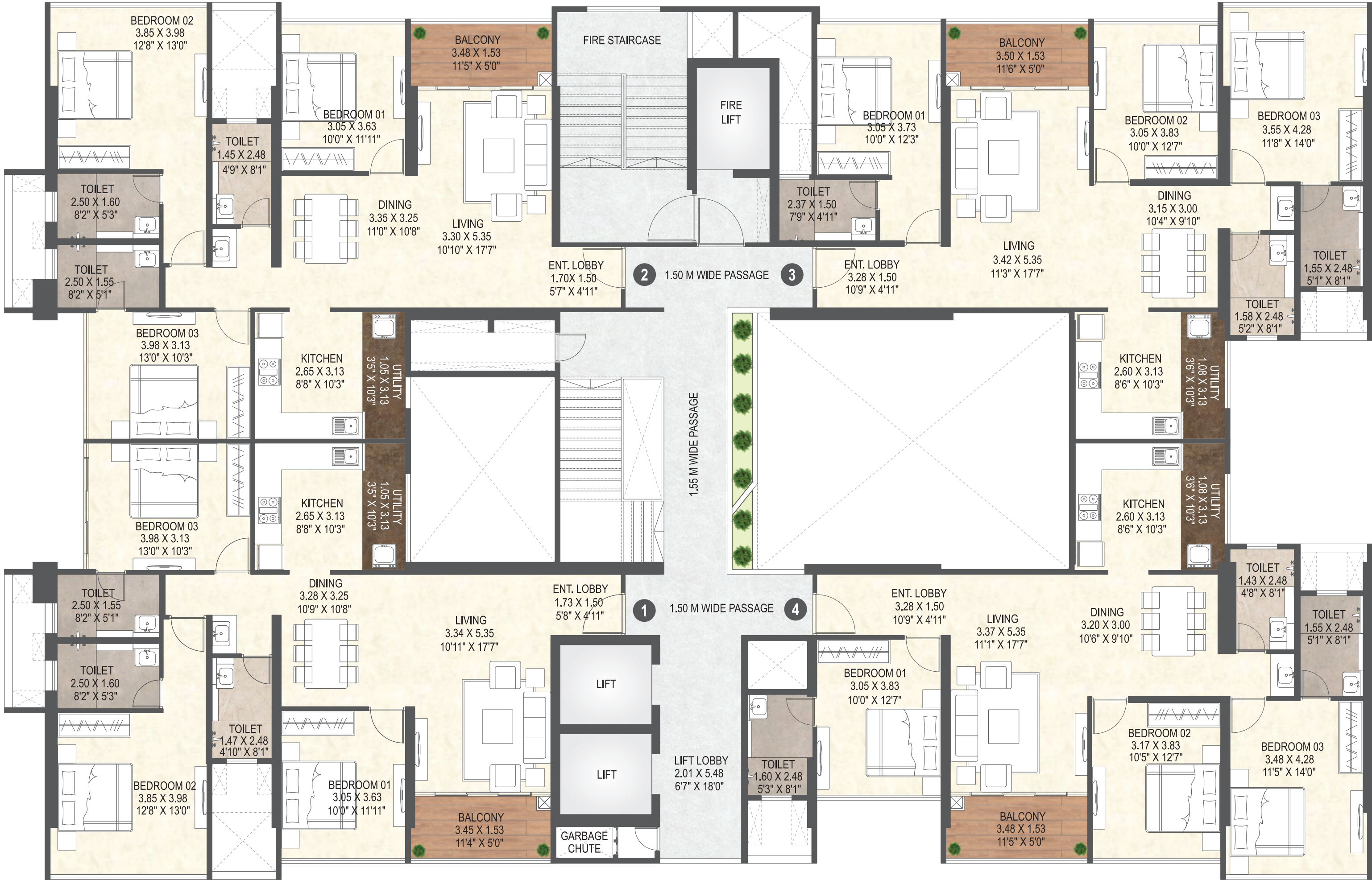
TYPICAL FLOOR PLAN: 2 ND , 4 TH , 5 TH , 6 TH , 7 TH , 9 TH , 10 TH , 11 TH , 12 TH , 14 TH , 15 TH , 16 TH , 17 TH , 19 TH , 20 TH , 21 ST , 22 ND & 23 RD
